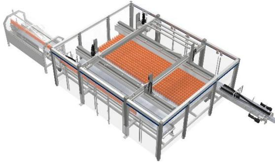
Figure 7 Polyketting accumulation conveyor
