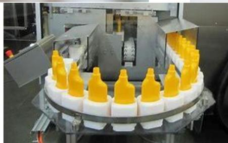
Many containers however are less complex as they are flat based, stable and easier to handle as shown below but due to the characteristics of the product being filled, i.e. highly viscous or containing solids, they are often filled at much lower speeds of between 8,000 – 15,000 containers per hour.
