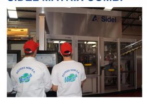
Following a significant investment in the biggest-ever Sidel Combi for CSD (carbonated soft drinks) in 2011, Refres Now, the Argentinian producer of the Manaos brand of beverages, has recently installed a further blow-fill-cap solution. With the new Sidel Matrix™ Combi, Refres Now can expect comparable savings of 45% in its energy consumption. It also anticipates a significant decrease in water consumption and an improvement of 40% in the plant's total production output.
